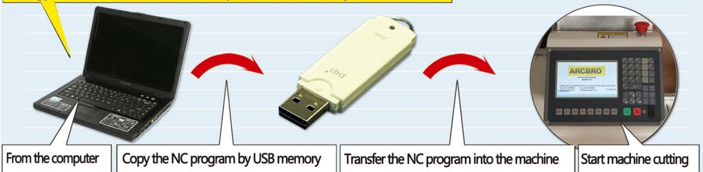
**Through USB Port ! Input and output the NC program simply.**
