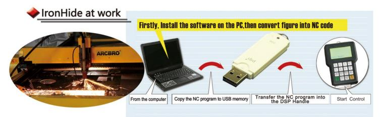
Through USB Port! Input and output the NC program simply.
